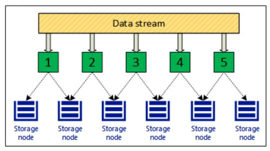
Replication in Acronis Storage is similar to the RAID rebuild process but has two key differences:
