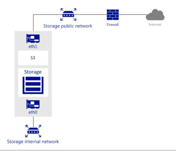
**Note:** In the scenario pictured above, the internal network is used for both the storage and S3 cluster traffic.
