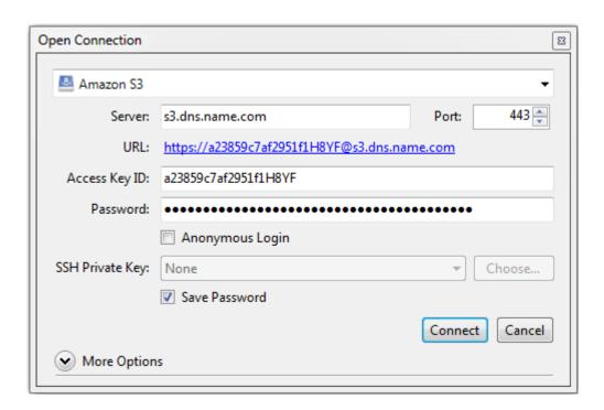
By default, the connection is established over HTTPS. To use CyberDuck over HTTP, you must install a special S3 profile from https://trac.cyberduck.io/wiki/help/en/howto/s3.
