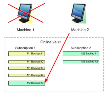
All earlier created backups remain intact. You can delete them manually if necessary. Keep in mind though, backups can be deleted from a subscription only by the machine to which the subscription is assigned. In our example, you have the following options.
