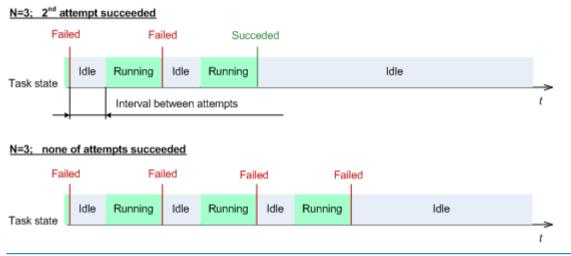
*If the task fails because of a mistake in the backup plan, you can edit the plan while the task is in the Idle state. While the task is running, you have to stop it prior to editing the backup plan.*
