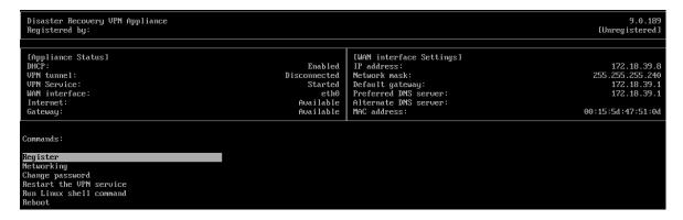
Make sure that the **IP address**, **Default gateway**, and **Preferred DNS server** settings are in place and correct. Note that the **Internet** and **Gateway** settings on the left side of the table must be **Available** for a successful appliance registration. Otherwise, please check your Default gateway and DNS availability settings before proceeding with registration or set the IP address manually.
