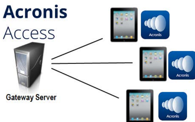
Fig 1. Single Gateway server, many Access Mobile Clients
