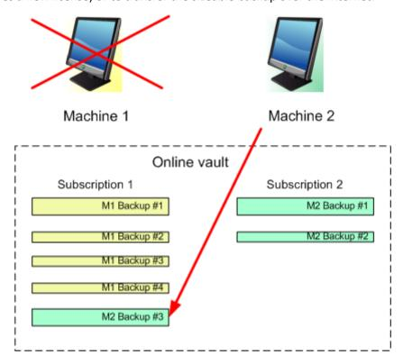
All earlier created backups remain intact. You can delete them manually if necessary. Keep in mind though, backups can be deleted from a subscription only by the machine to which the subscription is assigned. In our example, you have the following options.
